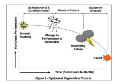
By using the 'tell-tale' evidence of changing equipment performance due to degradation, you can detect a failure and act to address it before an unplanned production disruption occurs. How soon
